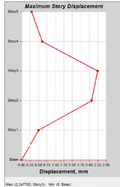
Fig.14 Story displacement of 150mm offset at partially filled condition
