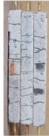
Fig 11. Crack pattern of polypropylene fibre reinforced UHPC
