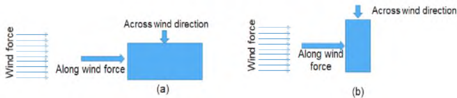
Fig 6. Different plan orientations of the building subjected to wind force (a) Long body, (b) Short body
