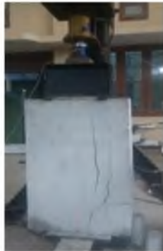
Figure 7: Failure mode of wall
