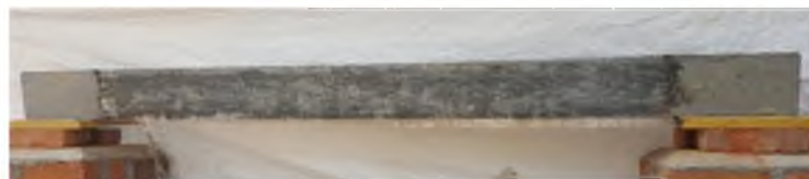
Fig 7. GFRP wrapped beam
