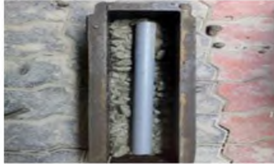
Fig 1: Beam with pipe
