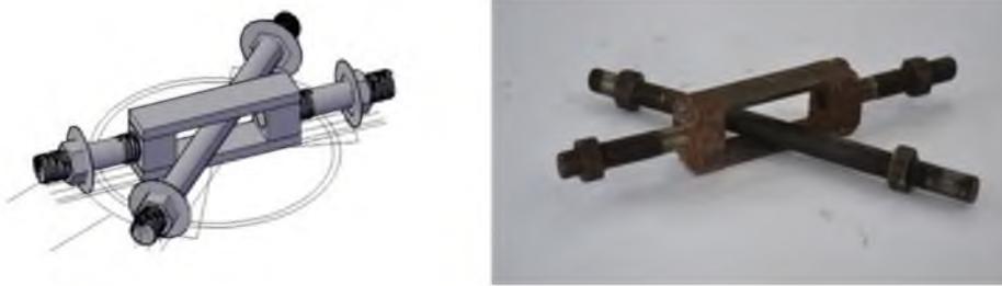
Fig.2. Split Bolt Assembly
