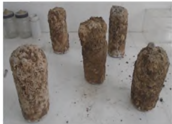
Fig 2. Exhumed columns in inverted position
