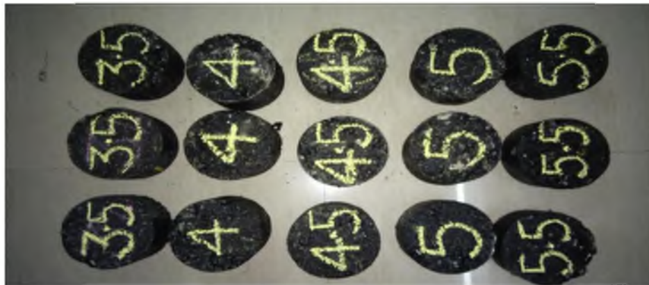
Fig 3.2 shows the Marshall samples that are prepared for the test of stability and flow for VG 30 samples of different Bitumen content
